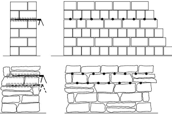
Example of bore hole arrangement – pressure injection
